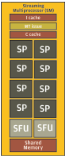
Figure 4: A single Streaming Multiprocessor (NVIDIA)
