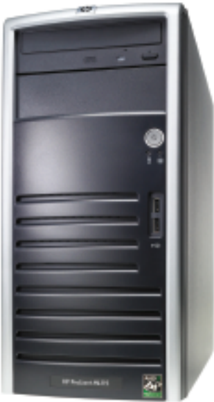
An HP ProLiant ML100 series entry-level server for light to moderate loads—a good file and database server
