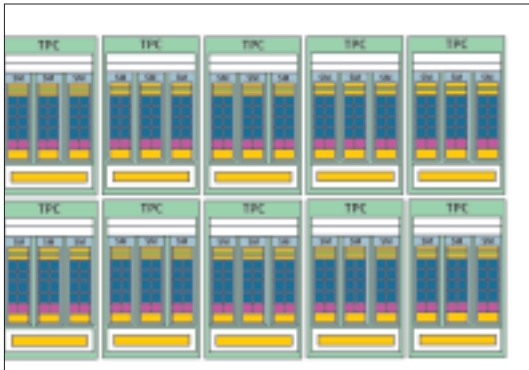
NVIDIA's GTX2xx architecture - 8 SPs combine to make 1 SM, 3 such SMs make up 1 TPC. 10 TPCs house 240 SPs in all.
